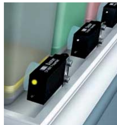
Liquid level monitoring (see box 10)
